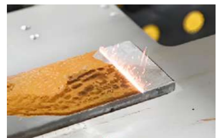
Dirty Laser Removing
